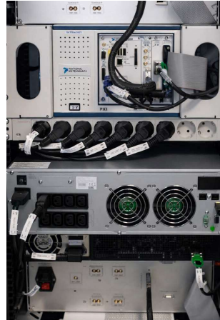
Data streaming and high-speed digital communications Validation system for the high-speed communication bus. PXI-based system. I/F electronic design for 1.5 Gbit/s HS bus. Data acquisition up to 3 terabytes. 6 test benches for DPU and VCU.
