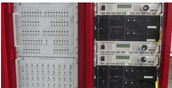
Hardware and software support bench for troubleshooting Detailed view of power racks.
