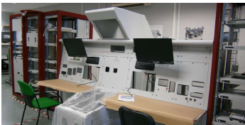
Hardware and software support bench for troubleshooting Cockpit simulator.
