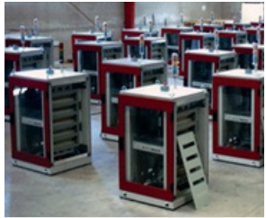
Interface test system for FAL (Final Assembly Line) Interconnection racks to connect the test systems with the aircraft
