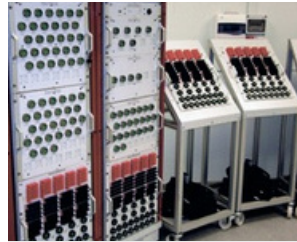
Interface test system for FAL (Final Assembly Line) These 39 equipments test different Aircraft's Electronics Subsystems
