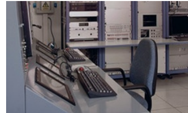
Integration rig for maritime patrol mission Console simulators
