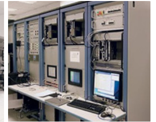
Integration RIG for P3-ORION Detailed view of the racks containing the mission equipments
