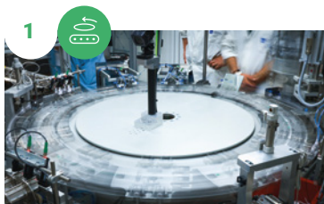
Fully automatic assembly machine with bowl feeders, robots and vision systems for lower cycle time operations.
