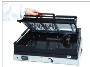
ICT Fixture for Aeroflex handler (vacuum, offline)
