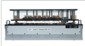
ICT fixture for EIIT ILS-1200 handler (pneumatic, inline)
