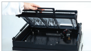
ICT fixture for Digital Test MTS-100 handler (vacuum, offline)
