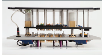
ICT fixture RF-20 handler (pneumatic, offline)
